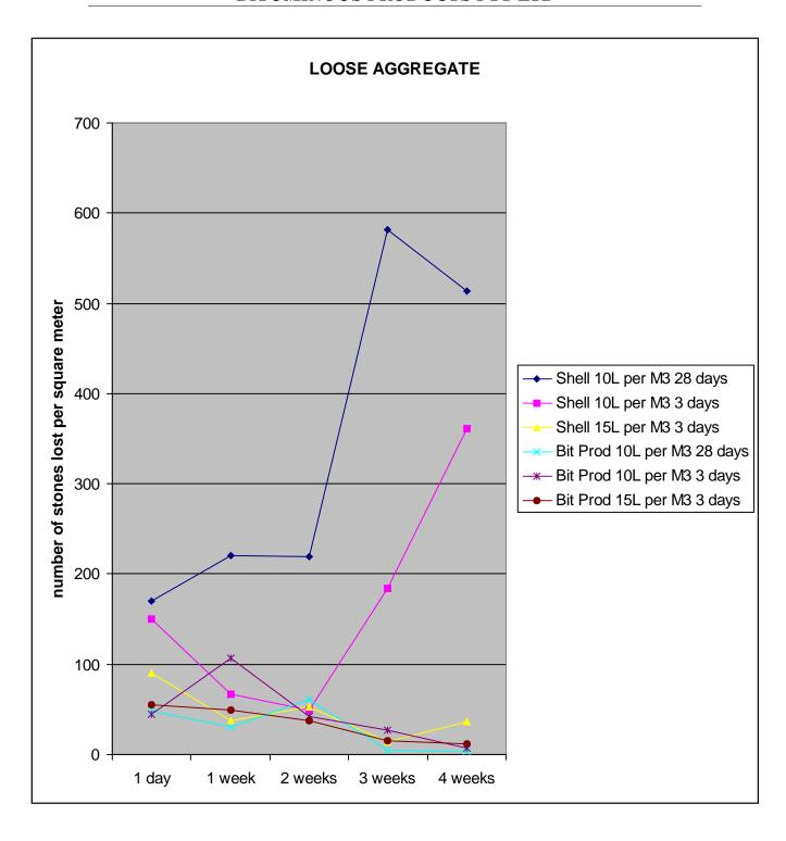
These are the results of a test conducted by Queensland Main Roads. Shell and Bituminous Products precoats were applied to 14mm Hornsfels at both the recommended rate of 10 litres per cubic meter and were stockpiled for 3 days and 28 days. They were also applied at 50% over the recommended rate at 15 litres per cubic meter and stockpiled for only 3 days.
